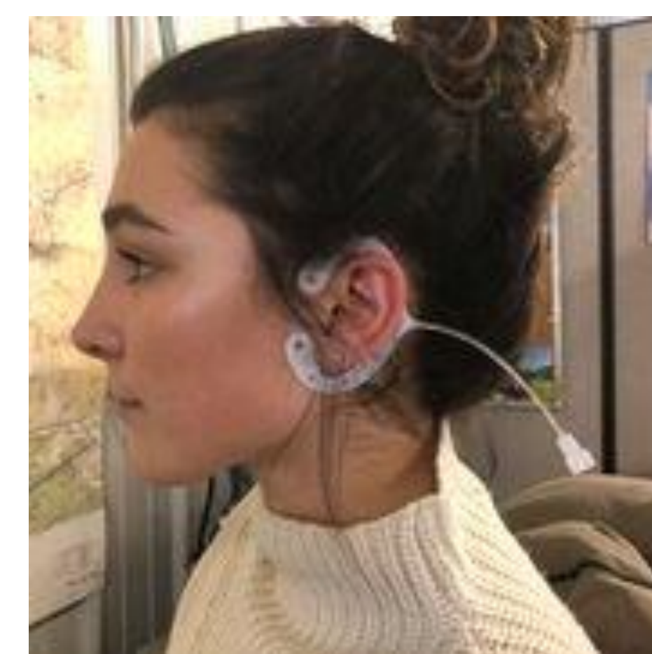
Figure 1. Subject wearing the cEEGGrid Array [6]
